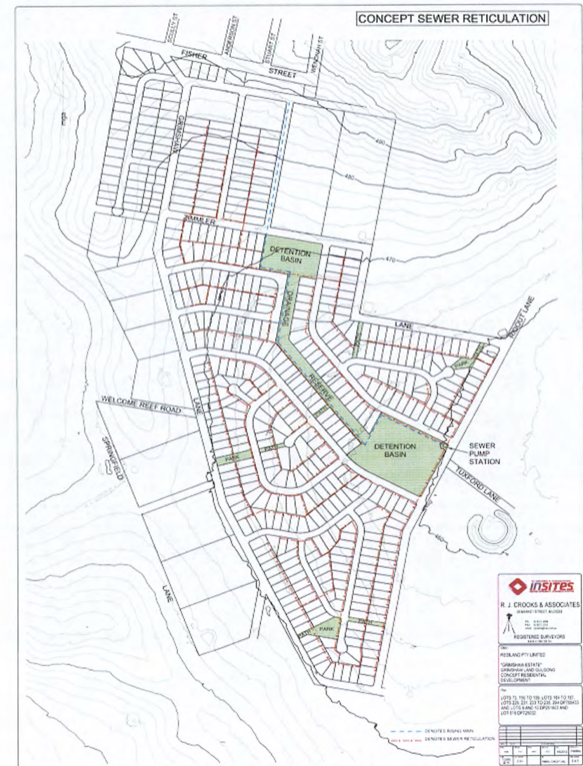
Figure 3.3: Concept Sewerage Reticulation
